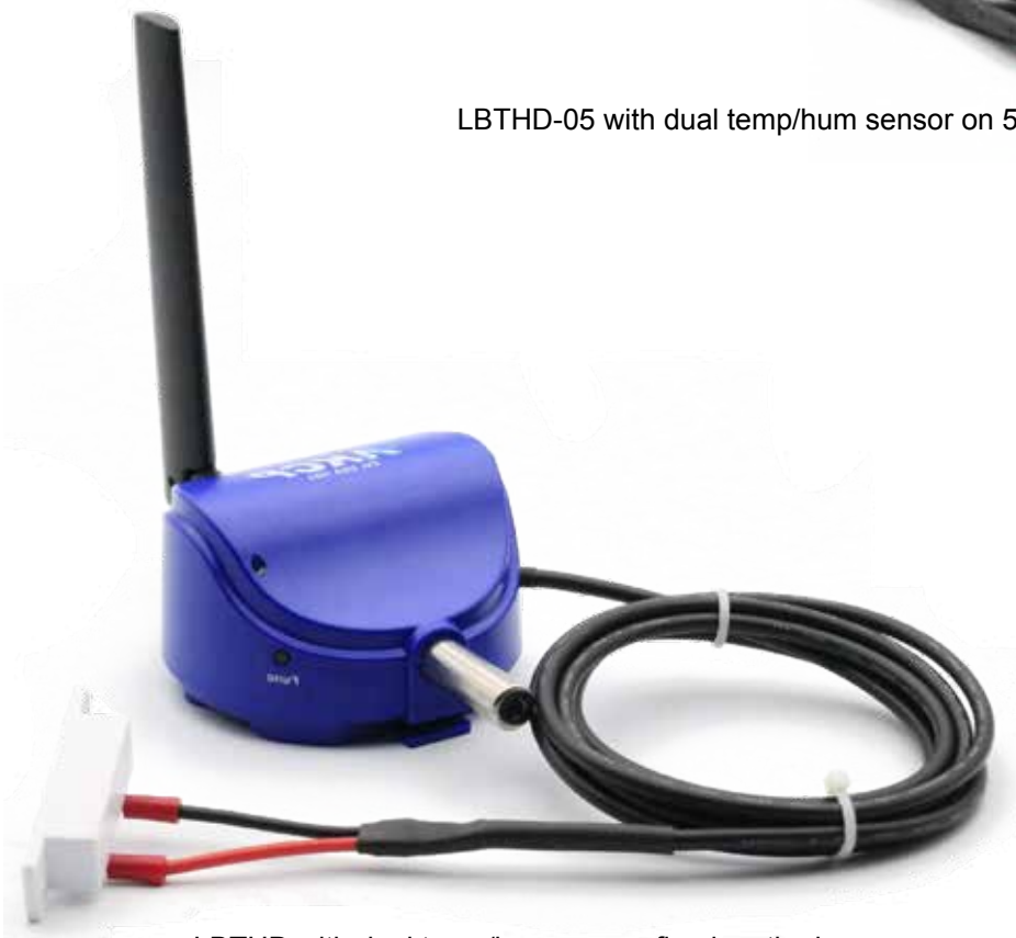
LBTHD with dual temp/hum sensor fixed on the box
