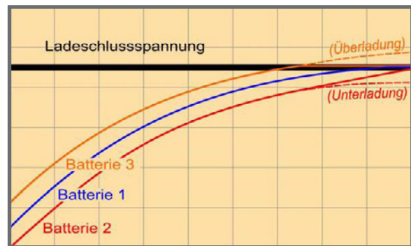
The charging of accumulators according to BACS® patented equalization process. The charging of Batterie 3 is capped to prevent overcharging and gassing. Supply of charging energy to Batterie 2 is continued and boosted until the target charging voltage is obtained. Batterie 1 performs ideally and is not regulated.
